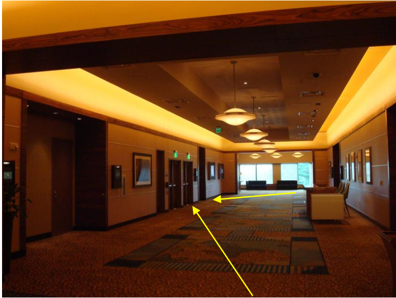
Exit Access: that portion of a means of egress that leads to an exit.
